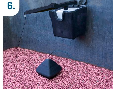
Place the anchor directly beneath the activation arm, pushing the anchor into the seed to secure it.
