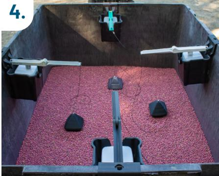
When installing multiple devices, place one on each side of the seed box, up to 4 total. Follow the rest of the directions for each device.
