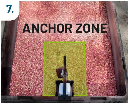
To ensure the CLIPS device works properly, the anchor must be placed under the activation arm and remain in the half of the seed box closest to the device, as represented by the anchor zone.
