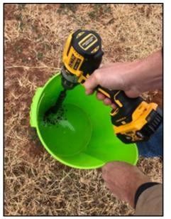
Figure 6.6: Soil Carbon sampling with drill auger.
