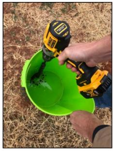
Figure 6.6: Soil Carbon sampling with drill auger.
