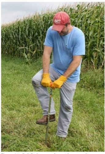
Figure 6.5: Soil Carbon sampling with step probe.
